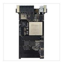
The Flexor™ 5973 is a high-performance 3U OpenVPX board based on the Xilinx Virtex-7 FPGA. As a stand-alone processor board, it provides an ideal development and deployment platform for demanding signal-processing applications.
