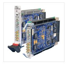
**The 52630 is a high-speed data converter, suitable for connection to HF or IF ports of a communications or radar system.** Its built-in data capture and playback features offer an ideal turnkey solution. It includes 1 GHz A/D and D/A converters and four banks of memory. It features built-in support for PCI Express over the 3U VPX backplane.
