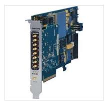
Model 7070-313 is a member of the Flexor® family of highperformance PCle boards based on the Xilinx Virtex-7 FPGA. As a
