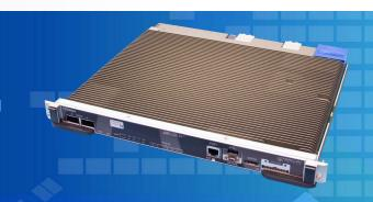
The rugged EnsembleSeries™ FCN8604 blade combines the general purpose processing capabilities of the EnsembleSeries HDS8613 with FPGA co-processing from dual Intel Arria 10 devices. By combining I/O, FPGA co-processing and general-purpose Intel processing in a single AdvancedTCA® blade, Mercury delivers a uniquely capable architecture for sensor processing in the open standard ATCA architecture.
