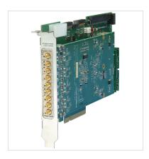
The Model 7891 generates up to eight synthesized clock signals suitable for driving A/D and D/A converters in high-performance real-time data acquisition and software radio systems. The clocks offer exceptionally low phase noise and jitter to preserve the signal quality of the data converters. These clocks are synthesized from onboard quad VCXOs (voltage controlled oscillators) and can be phase-locked to an external reference signal.
