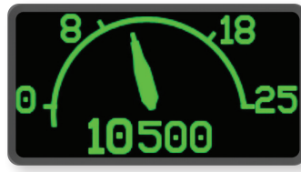
DIGITAL ALTITUDE WITH ANALOG-STYLE GAUGE SHOWING ALTITUDE TREND.
