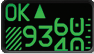
DIGITAL ALTITUDE WITH ROLLING DIGITS AND ALTITUDE TREND MARKER.
