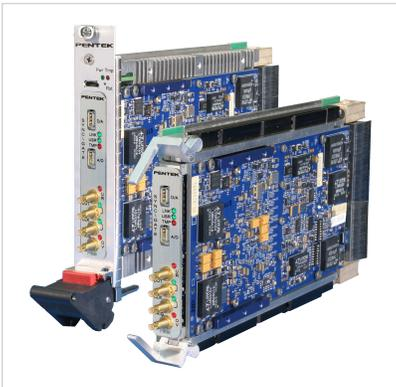
**The 52630 is a high-speed data converter, suitable for connection to HF or IF ports of a communications or radar system.** Its built-in data capture and playback features offer an ideal turnkey solution. It includes 1 GHz A/D and D/A converters and four banks of memory. It features built-in support for PCI Express over the 3U VPX backplane.
