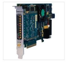
Model 7070-316 is a member of the Flexor® family of highperformance PCle boards based on the Xilinx Virtex-7 FPGA. As a FlexorSet® integrated solution, the Model 3316 FMC is factory-installed on the 7070 FMC carrier. The required FPGA IP is installed and the board set is delivered ready for immediate use.
