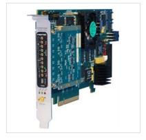
Model 7070-324 is a member of the Flexor® family of high-performance PCle boards based on the Xilinx Virtex-7 FPGA. As a FlexorSet™ integrated solution, the Model 3324 FMC is factory-installed on the 7070 FMC carrier. The required FPGA IP is installed and the board set is delivered ready for immediate use.
