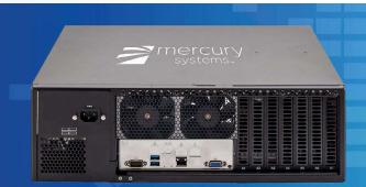
Engineered to handle massive workloads anywhere, Mercury's *EnterpriseSeries* RES AI 3U server employs the latest NVIDIA® Tesla® GPUs and Intel® Xeon® Scalable processors to accelerate compute-heavy mission-critical applications such as Signal Intelligence (SIGINT), cryptography, deep learning, Artificial Intelligence (AI), surveillance, sensor fusion, visualization, image processing, tracking and big data analytics.
