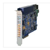
The 78670 is a 4-channel, high-speed data converter, suitable for connection to HF or IF ports of a communications or radar system. Its built-in data playback features offer an ideal turnkey solution for demanding transmit applications.
