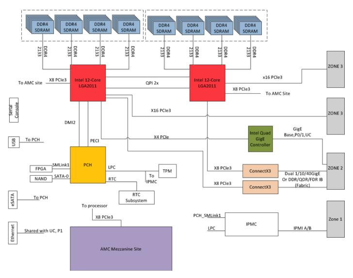
Figure 1 - EnsembleSeries HDS8613 Functional Block Diagram
