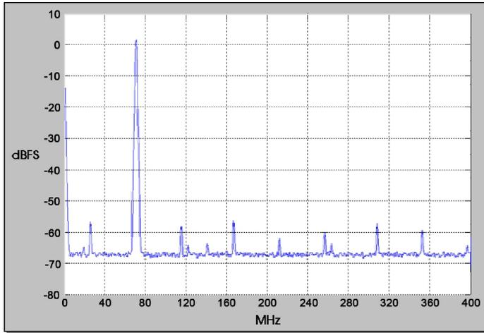
$f_{out} = 70 \text{ MHz}$ ,  $f_s = 800 \text{ MHz}$ , Interpolation = 4,
