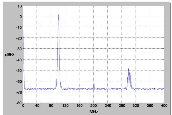
$f_{out} = 100 \text{ MHz}$ ,  $f_s = 800 \text{ MHz}$ , Interpolation = 4,
