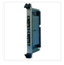
The 57741 and the 58741 consist of one or two 71741 XMC modules mounted on a 6U VPX carrier board. The 57741 is a 6U board with one 71741 module while the 58741 is a 6U board with two XMC modules rather than one.
