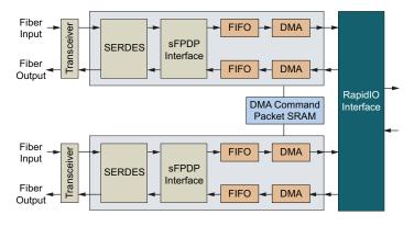
Figure 1. XMC Channel block diagram
