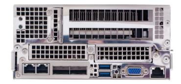
Weight\*\*\*: 12.5 lb. (5.67 kg), 15 lb. (6.80 kg) with TESLA card Expansion: up to 5 PCle Cards
