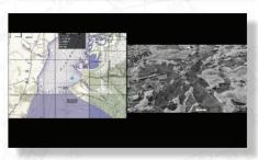
Like split screen, picture-by-picture or side-by-side displays two inputs next to each other; these images, however, retain the aspect ratios of their respective video inputs. Excess screen space appears as black bars.
