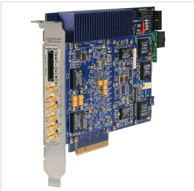
**The 78650 is a multichannel, high-speed data converter, suitable for connection to HF or IF ports of a communications or radar system.** Its built-in data capture and playback features offer an ideal turnkey solution. It includes two A/Ds, one DUC (Digital Upconverter), two D/As, and four banks of memory.
