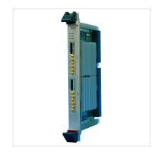
Models 57651 and 58651 consist of one or two 71651 XMC modules mounted on a VPX carrier board. The 57651 is a 6U board with one 71651 module while the 58651 is a 6U board with two XMC modules rather than one.
