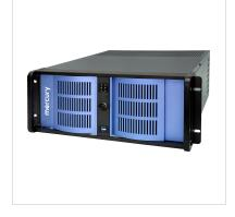
The Talon® RTR 2749 is a turnkey system, used for recording high-bandwidth signals. The RTR 2749 uses 12-bit, 3.6 GHz A/D converters. It can be configured as a one- or two-channel system and can record sampled data, packed as 8-bit- or 16-bit-wide consecutive samples (12-bit digitized samples residing in the 12 MSBs of the 16-bit word). A high-speed RAID array provides a maximum streaming recording rate to disk of 4.8 GB/sec.
