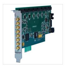
The 7893 System Synchronizer and Distribution Board synchronizes multiple Mercury Cobalt and Onyx boards within a system. It enables synchronous sampling, playback and timing for a wide range of multichannel high-speed data acquisition, DSP and software radio applications.
