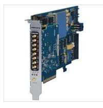
**Model 7070-312 is a member of the Flexor® family of highperformance PCIe boards based on the Xilinx Virtex-7 FPGA.** As a FlexorSet® integrated solution, the Model 3312 FMC is factory-installed on the 5973 FMC carrier. The required FPGA IP is installed and the board set is delivered ready for immediate use.
