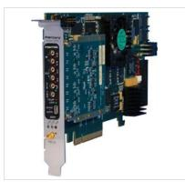
Model 7070-320 is a member of the OnyxFX® family of highperformance PCIe baseboards with a Xilinx Virtex-7 FPGA and an available FMC I/O slot. As an integrated solution, the Model 7070-320 FlexorSet® combines the Model 7070 and the Model 3320 Flexor® FMC as a factory-installed set. The required FPGA IP is installed and the board set is delivered ready for immediate use.
