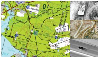
Quad vertical mode displays input signals as one large and three small images along left or right side of display.
