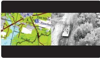
Picture-by-picture (PBP), or side-by-side mode, displays two input signals next to each other as equally-sized images whose aspect ratios are maintained. Excess screen space appears as black bars.
