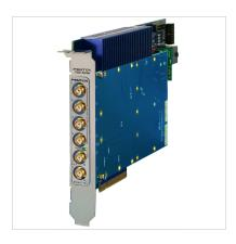
The 7894 High-Speed Clock Generator provides fixed-frequency sample clocks to Cobalt and Onyx PCle boards in multi-board systems. It enables synchronous sampling, playback and timing for a wide range of multichannel high-speed data acquisition and software radio applications.
