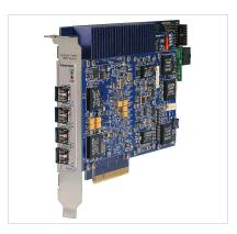
The 78611 is a multichannel, gigabit serial interface, ideal for interfacing to Serial FPDP data converter boards or as a chassisto-chassis data link. The 78611 is fully compatible with the VITA 17.1 Serial FPDP specification. Its built-in data transfer features make it a complete turnkey solution. For users who require application-specific functions, the 78611 serves as a flexible platform for developing and deploying custom FPGA processing IP.
