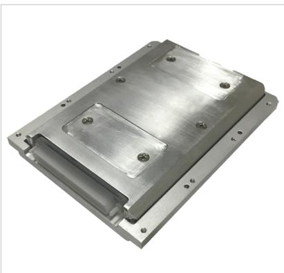
**The JDAR is a miniature, Type-1 certified, rugged data-at-rest inline encryption solution that stores and protects Secret and Below (SAB) data.** Flexible, compact, and fast, it can be integrated into existing systems or used as a standalone encryption device for avionics and unmanned platforms, as well as unattended sensors, surveillance, communication, and wearable systems.
