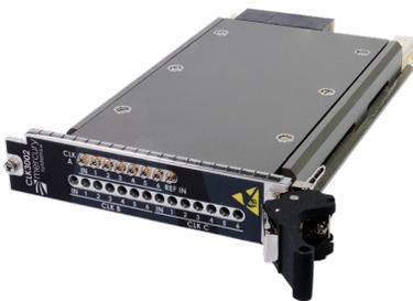
Our clock technology incorporates a modular design approach to enable rapid factory customization. This flexible architecture also includes multiple coherent outputs in a convenient OpenVPX form factor. Ideal for applications such as direction finding and digital beam forming that require multiple coherent clock channels all operating with minimal jitter, this modular clock technology provides the high-fidelity performance for next-generation systems.
