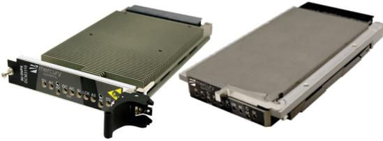
Our EnsembleSeries™ IF processing and direct conversion solutions enable the real-time digitization and processing of complex signals. We integrate the most advanced ADC, DAC and FPGA technology in 3U and 6U OpenVPX™ modules to create a product portfolio to support applications such as electronic warfare, spectrum monitoring and digital beam steering.
