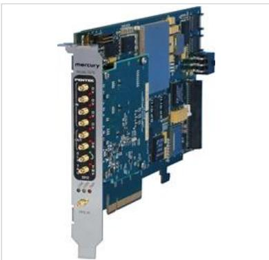
**The Flexor® Model 7070 is a high-performance PCIe board based on the Xilinx Virtex-7 FPGA.** As a stand-alone processor board, it provides an ideal development and deployment platform for demanding signal processing applications.
