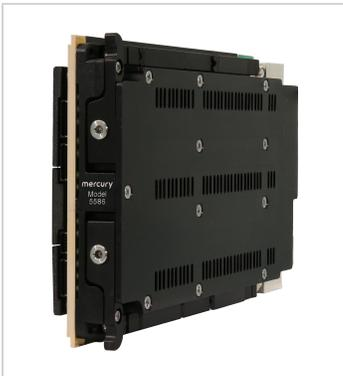
**The 5586 is a high-performance, SOSA aligned 3U OpenVPX co-processor board based on the Xilinx Virtex UltraScale+ HBM FPGA.** It serves as an ideal stand-alone processor or as a co-processor for distributed FPGA processing tasks.
