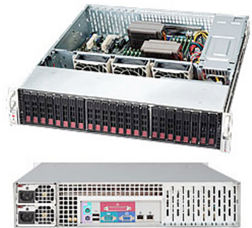
Figure 2 - An example of a commercial Storage Target subsystem
