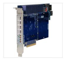
The Model 7892 High-Speed Synchronizer and Distribution PCle Board synchronizes multiple Cobalt, Onyx, Flexor, or Jade boards within a system. It enables synchronous sampling and timing for a wide range of multichannel high-speed data acquisition, DSP, and software radio applications. Up to four boards can be synchronized using the 7892, with each receiving a common clock along with timing signals that can be used for synchronizing, triggering and gating functions.
