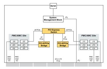
Figure 1. CCM6020 Module block diagram
