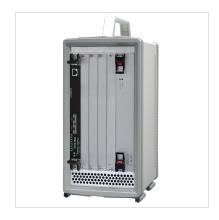
The 8258 is a low-cost 6U VPX development platform ideal for developing applications on Mercury's SCFE6931 heterogeneous processing module. Providing power and cooling to match the SCFE6931 in a small desktop footprint, the chassis allows access to all required interfaces on the SCFE6931 front panel. The 8258 can be configured with up to eight optional MPO optical connectors to support the 100 GigE interfaces on the SCFE6931 module.
