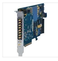
The Flexor<sup>®</sup> Model 7070 is a high-performance PCIe board based on the Xilinx Virtex-7 FPGA. As a stand-alone processor board, it provides an ideal development and deployment platform for demanding signal processing applications.
