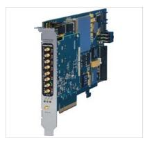
Model 7070-313 is a member of the Flexor® family of highperformance PCle boards based on the Xilinx Virtex-7 FPGA. As a
