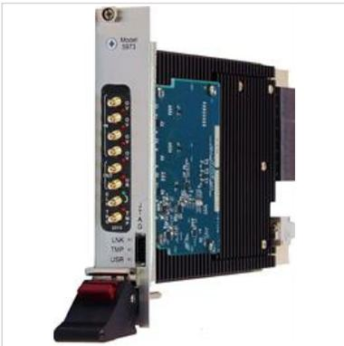
**Flexor® 5973-312 is a member of the Flexor family of high-performance 3U VPX boards based on the Xilinx Virtex-7 FPGA.** As a FlexorSet® integrated solution, the 3312 FMC is factory-installed on the 5973 FMC carrier. The required FPGA IP is installed and the board set is delivered ready for immediate use.
