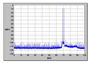
$f_1 = 69 \text{ MHz}, f_2 = 71 \text{ MHz}, f_s = 200 \text{ MHz}$
