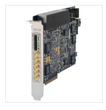
The 78761 is a multichannel, high-speed data converter with programmable DDCs (digital downconverters), suitable for connection to HF or IF ports of a communications or radar system.
