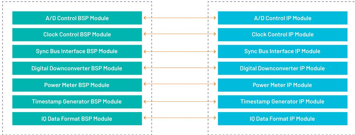
Because all Jade boards are shipped with a full suite of built-in IP functions and numerous software examples, new applications can be developed by building on the provided software examples or built entirely new with the BSP extensive libraries. All BSP libraries are provided as C-language source for full access and code transparency.
