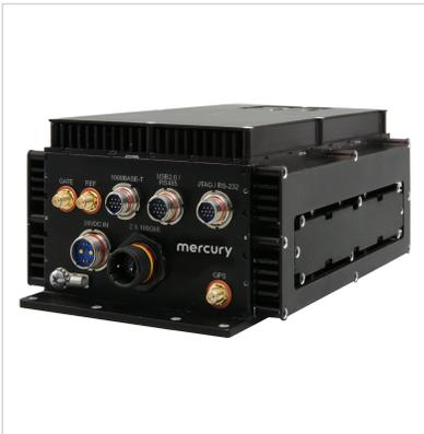
**The Quartz<sup>®</sup> 6350 is a high-performance, small form factor system based on the Xilinx Zynq UltraScale+ RFSoc.** The RFSoc integrates eight RF-class A/D and D/A converters into the Zynq's multiprocessor architecture, creating a multichannel data conversion and processing solution on a single chip.
