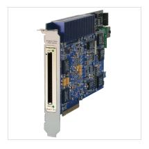
The 78610 digital I/O board provides 32 LVDS differential inputs or outputs plus LVDS clock, data valid, and data flow control on a front panel 80-pin connector. Its built-in data capture and data generation feature offers an ideal turnkey solution as well as a platform for developing and deploying custom FPGA-processing IP.
