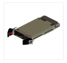
Increase multi-domain operation capabilities, while maintaining tight SWaP budgets. The dense combination of high performance CPU and FPGA processing technologies provides a highly versatile multifunction processing building block for radar, electronic warfare, and mission applications with tight SWaP requirements.
