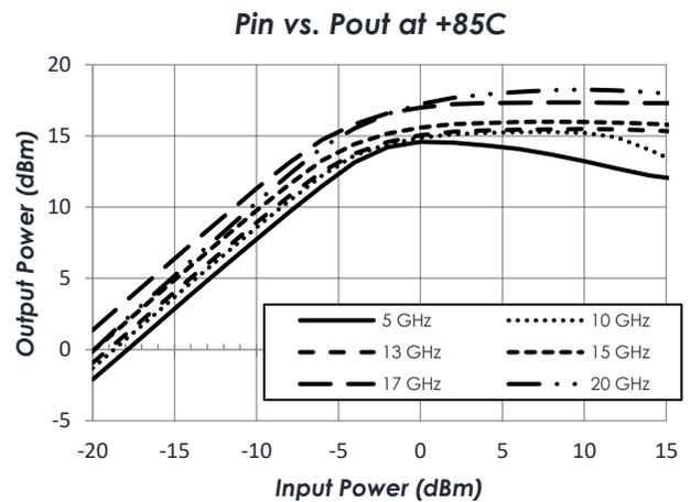
(Amplifier Bypass, VDD = VDD1 = VDD2 = VSW = +3.3 V, ID = 1 mA)
