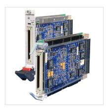
The 52610 digital I/O board provides 32 LVDS differential inputs or outputs plus LVDS clock, data valid, and data flow control on a front panel 80-pin connector. Its built-in data capture and data generation feature offers an ideal turnkey solution as well as a platform for developing and deploying custom FPGA-processing IP.
