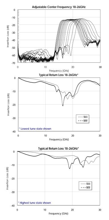
\* Typical values shown for lowest tuned frequency (control bits 0000) or highest tuned frequency (control bits 1111)
