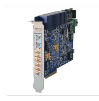
The 78671 is a 4-channel, high-speed data converter, suitable for connection to HF or IF ports of a communications or radar system. Its built-in data playback features offer an ideal turnkey solution for demanding transmit applications.
