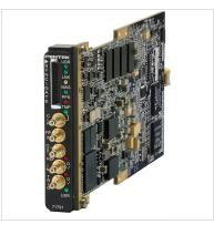
The 71791 is a L-band RF tuner, suitable for connection directly to an L-band signal for SATCOM and communications systems. Its built-in data capture features offer an ideal turnkey solution as well as a platform for developing and deploying custom FPGA processing IP.
