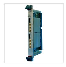
The 57690 and 58690 consist of one or two 71690 XMC modules mounted on a VPX carrier board. The 57690 is a 6U board with one 71690 module while the 58690 is a 6U board with two XMC modules rather than one.
