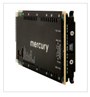
The 5560 is a high-performance, SOSA aligned 3U OpenVPX coprocessor board based on the AMD Versal™ HBM ACAP (Adaptive Compute Acceleration Platform). It serves as an ideal stand-alone processor or as a co-processor for distributed ACAP processing tasks.
