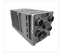
JARVIS (Joint Avionics Reconfigurable Virtual Information System) is a FACE™ 3.0 conformant, Integrated Modular Avionics 2nd generation (IMA-2G) architecture-based mission computer that dynamically allocates application resources across four common, reconfigurable, encrypted and networked computing modules to reduce downtime, risk and maintenance costs.
