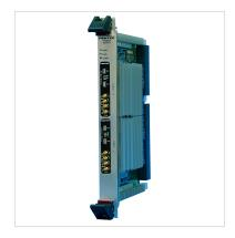
The 57730 and the 58730 consist of one or two 71730 XMC modules mounted on a VPX carrier board. The 57730 is a 6U board with one 71730 module while the 58730 is a 6U board with two XMC modules rather than one.
